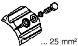
Fig.8 Electrical connection for earthing conductor
