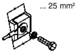
Fig.7 Electrical connection wherever terminal clips are used.
